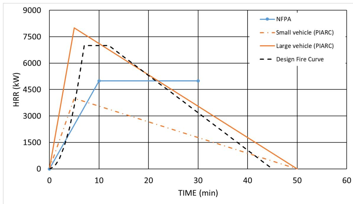
Figure 7 New design fire curve in comparison to design fires from other standards [12, 13]
