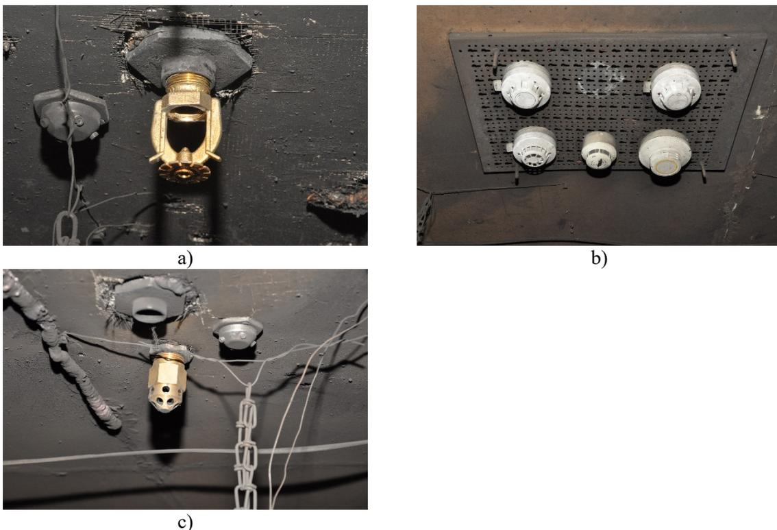
Figure 12 Photos of different parts of the systems used in the second fire test series: a) sprinkler head, b) different detection systems installed, c) nozzle for gaseous agents.
