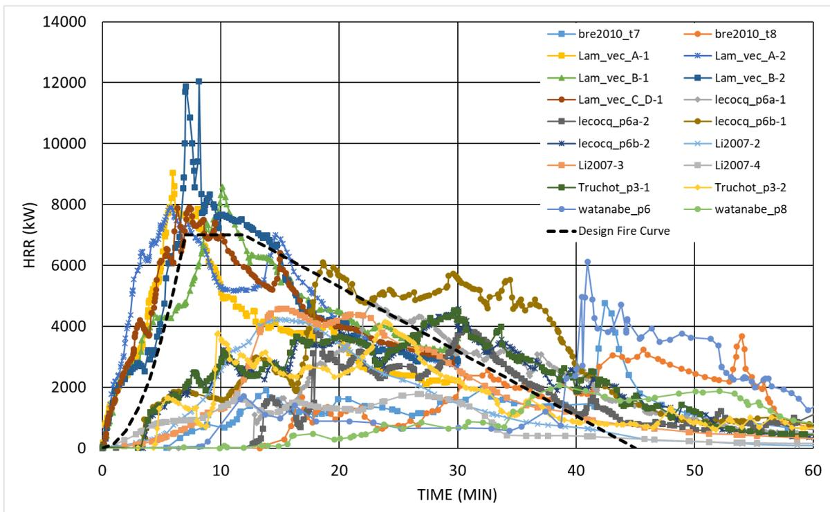
Figure 6 Comparison of new design fire curve and test data from literature
