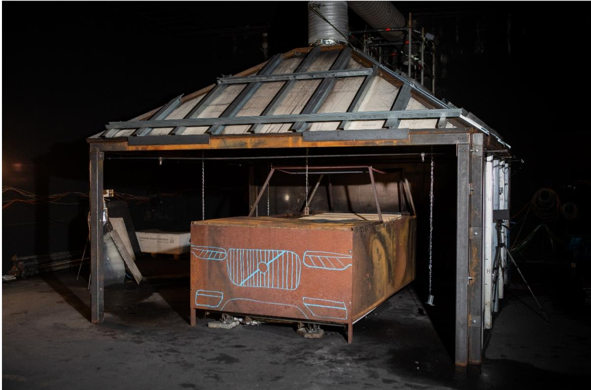
Figure 9 Calorimeter with vehicle mock-up and wooden design fire load
