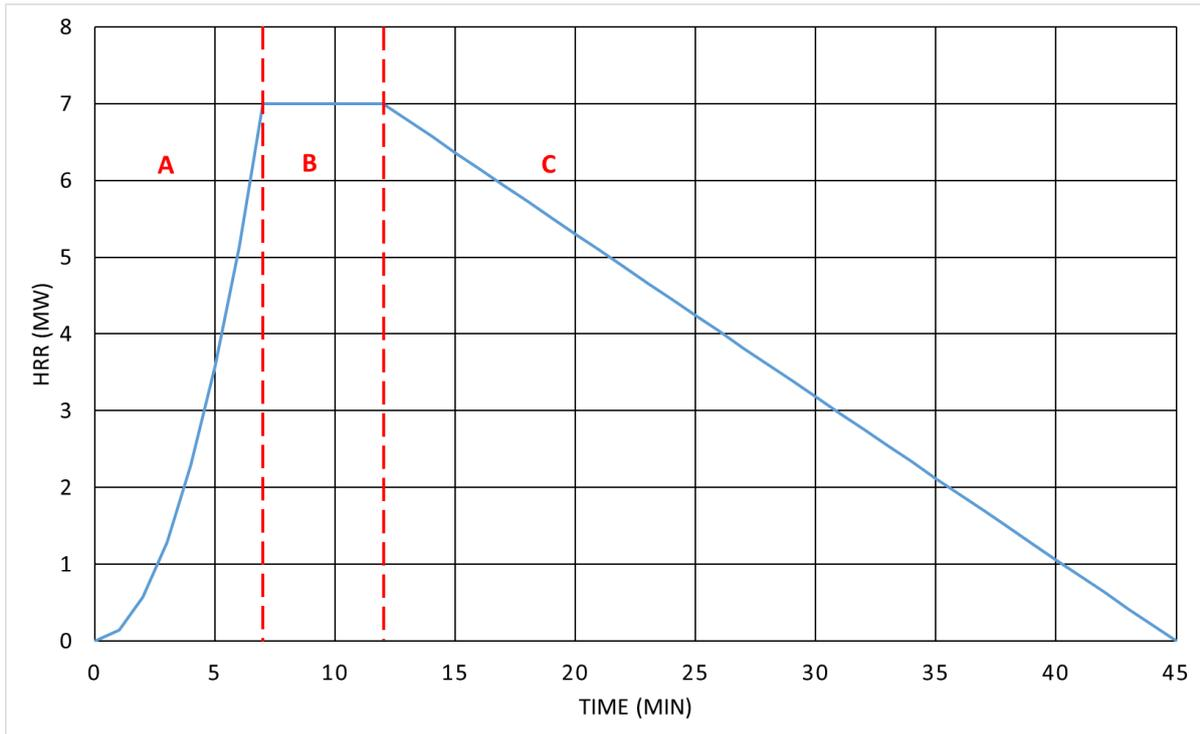
Figure 5 Design fire curve for ICE and electric vehicles
