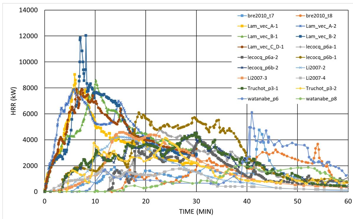
Figure 4 Collection of vehicle fire test data (HRR) with different ICE and battery vehicles based on literature studies [5, 6, 7, 8, 9, 10, 11]
