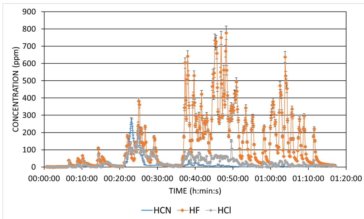
Figure 11 Gas concentrations of HCN, HF, and HCl measured during the 24 kWh battery fire test including error indicators.
