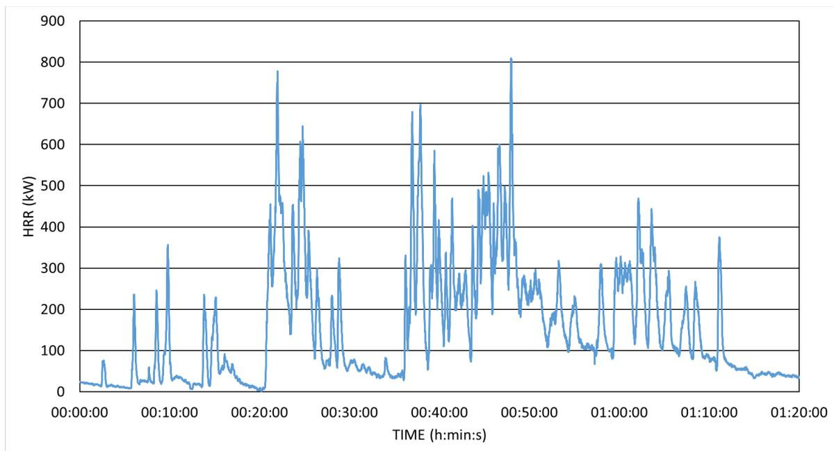
Figure 10 Heat Release Rate of 24 kWh battery pack determined by OCC
