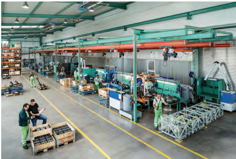
Fig. 10: Refurbishment at the Herrenknecht headquarters Up to 50 cutter experts in Schwanau handle the professional refurbishing of the disc cutters. In total an estimated 24,000 disc cutter changes are necessary for the 4 TBMs.
