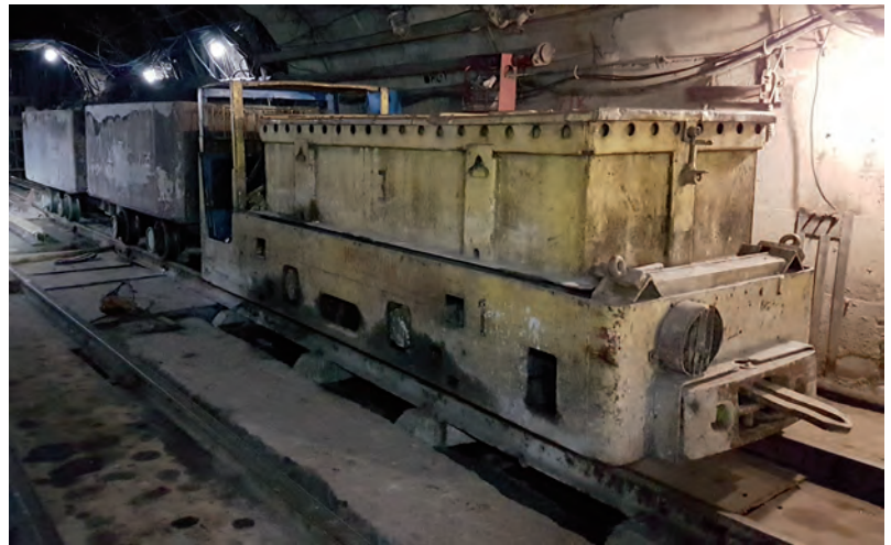
Fig. 4: Locomotives and mine cars deployed at the Donskoy GOK mine for transporting loaded muck Source: TOO Schachtbau Kasachstan
