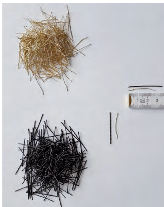
Fig. 12: Geometry of the fibres – made of steel above and polymer below
