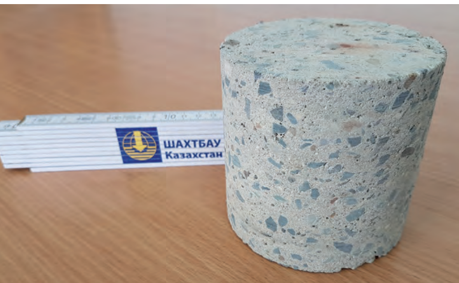
Fig. 11: Concrete core with 100 mm diameter and 100 mm in height prepared for concrete test – taken from shotcrete shell produced underground Source: TOO Schachtbau Kasachstan
