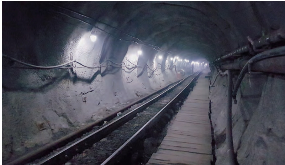
Fig. 14: Completely developed roadway including capital track and water channel (otr, covered)
