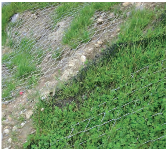
Fig. 9: Test area approx. 10 weeks after the hydro-seeding process and after heavy rain: otl without erosion control mat and otr with geomat
