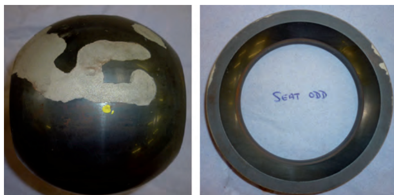
Fig. 1: Loss of the coating on the ball and the seat of the ball valve
