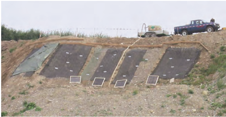
Fig. 8: Test areas in Switzerland for examining the efficacy of a geomat for erosion protection in 2013
