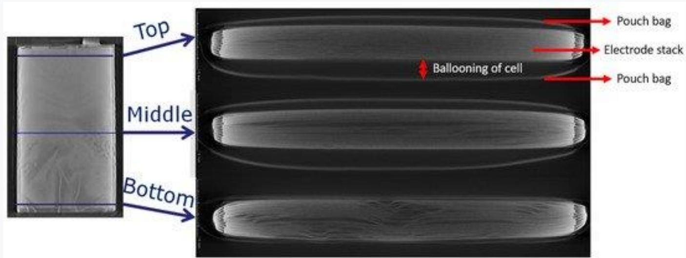
Picture: X-ray computed tomography cross-sections
