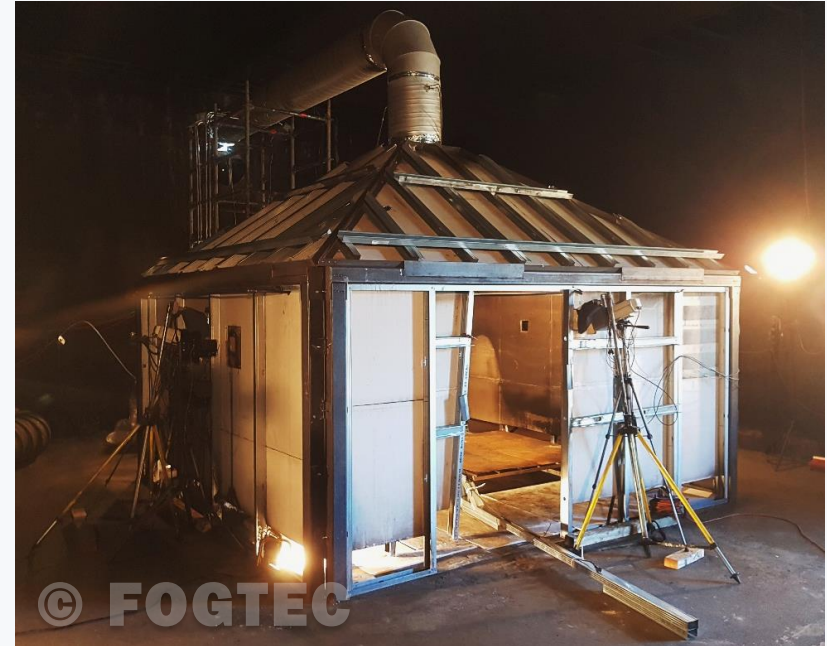
SUVEREN – Battery fire test chamber (calorimeter)
