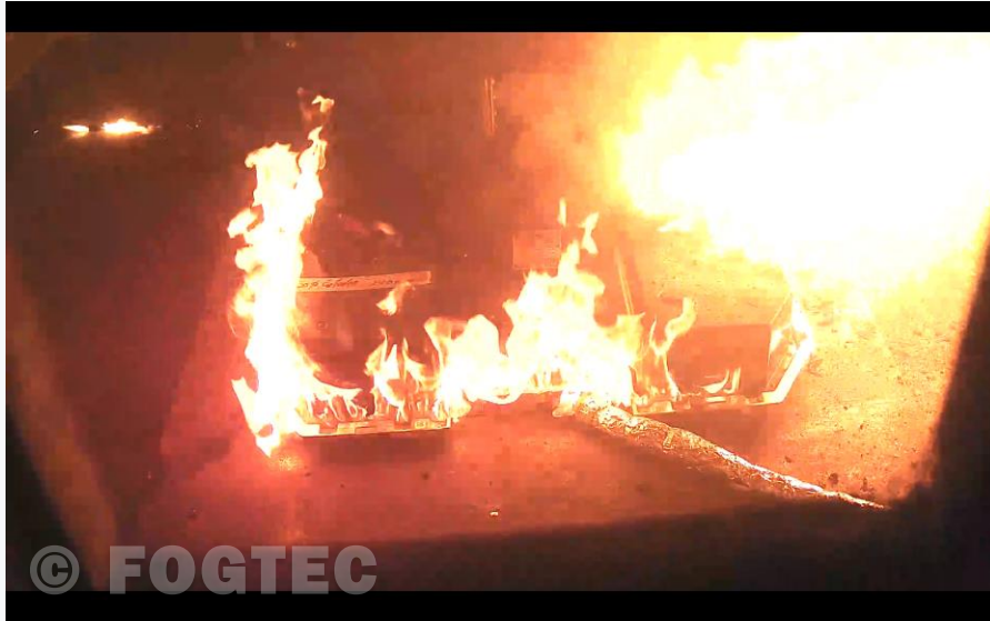
Figure: Fire test with vehicle lithium-ion batteries in the calorimeter
